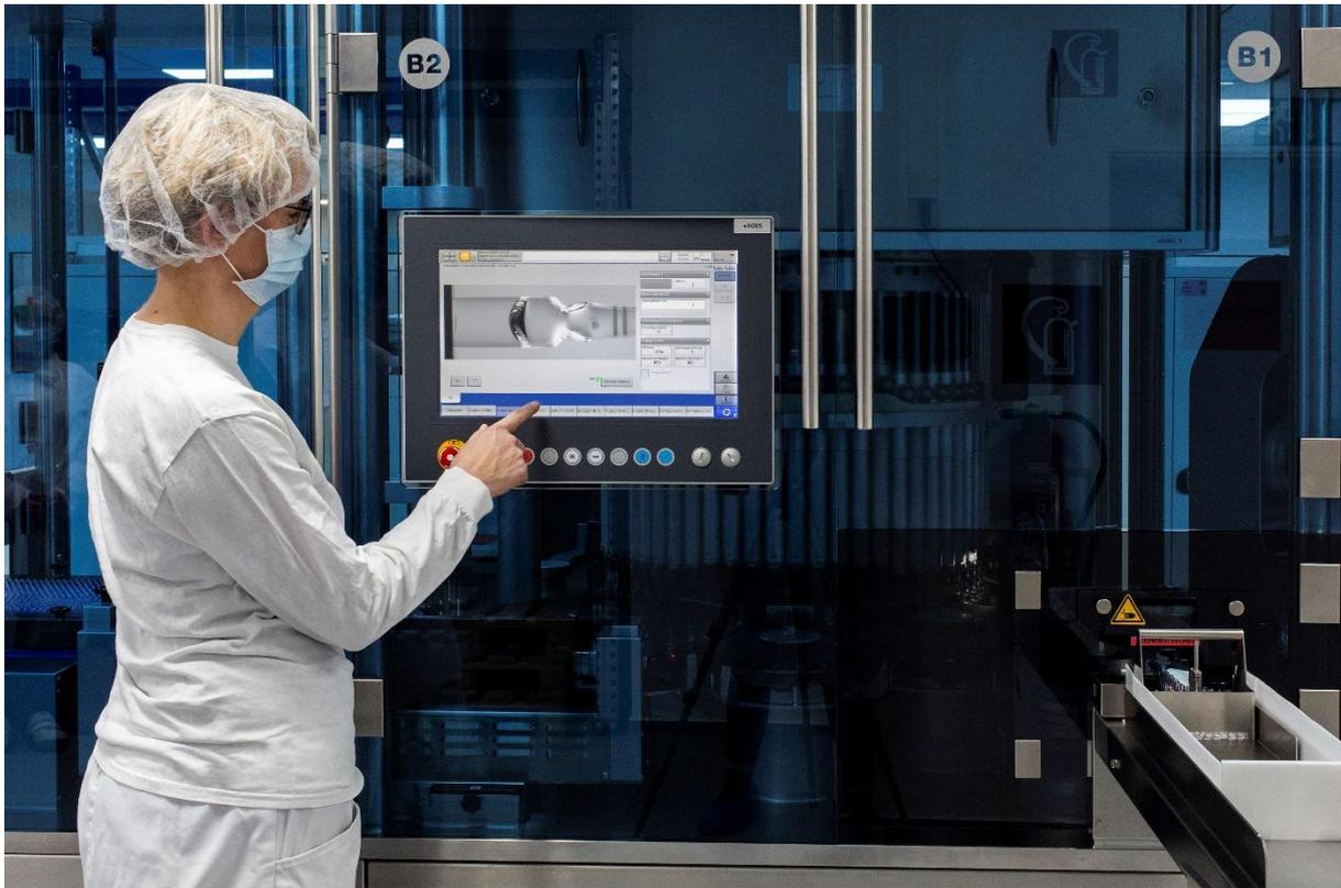
The new fully automatic optical inspection in liquid sterile production at Aenova in Gronau significantly increases controlled output. Operator starts the inspection process.
