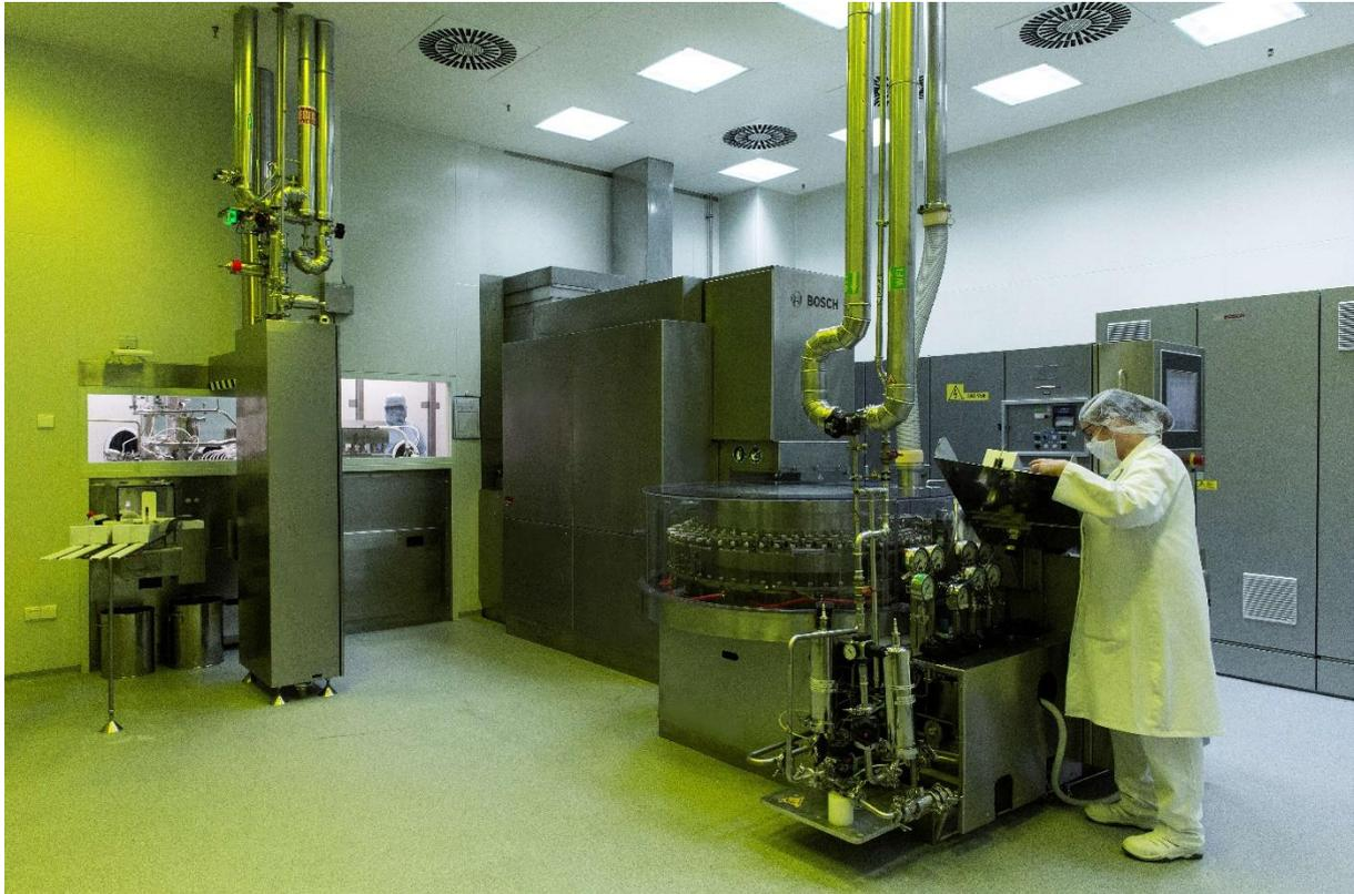
With the new sterile filling line, a total of 100 million ampoules and vials can be produced per year at Aenova in Gronau; here the cleaning and depyrogenation area. (Photo Aenova. Tanita Teichfischer).
