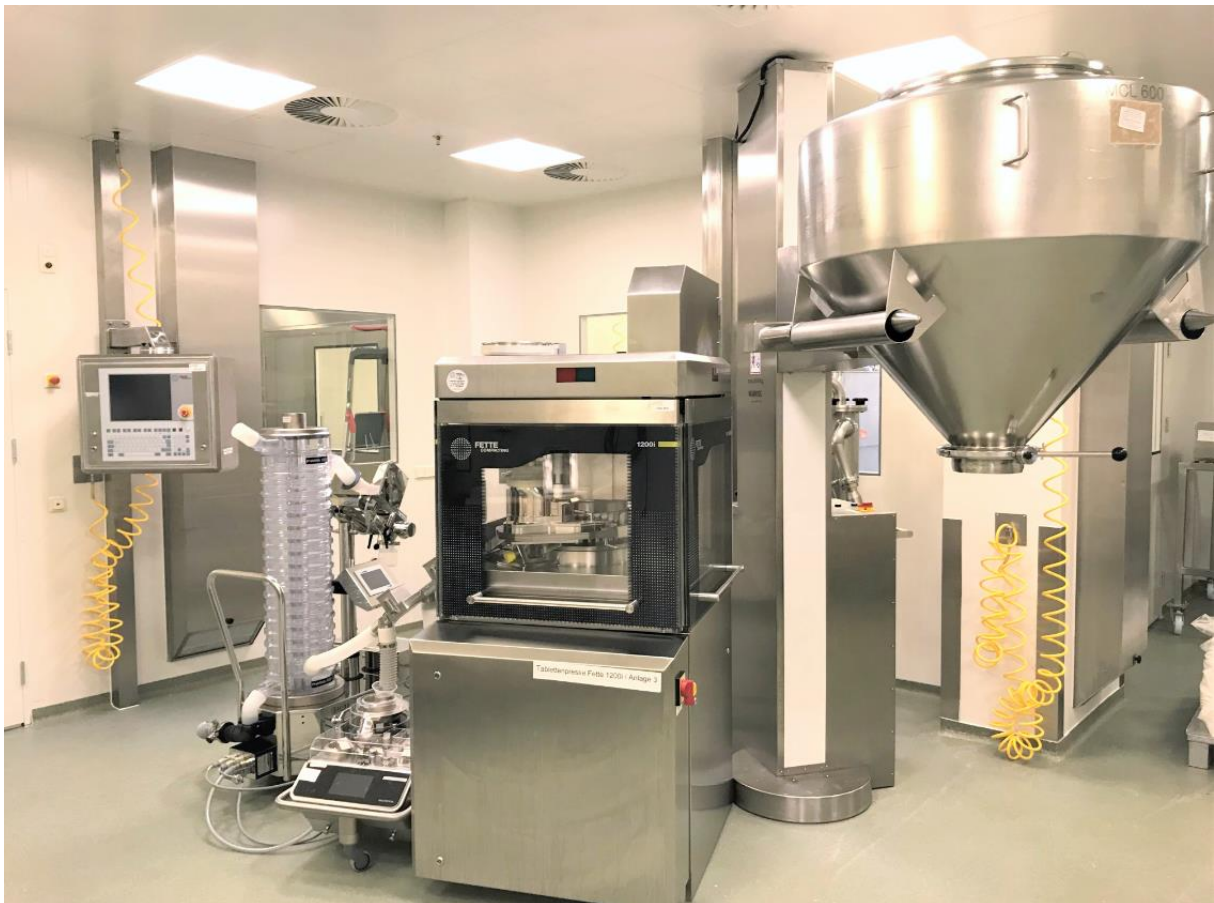
The new tablet press at Aenova in Regensburg for highly potent active ingredients enables flexible high containment production. (Photo: Aenova Group)
